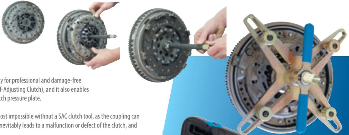
This SAC clutch tool kit is absolutely necessary for professional and damage-free removal and installation of SAC clutches (Self-Adjusting Clutch), and it also enables resetting of the SAC adjusting ring in the clutch pressure plate.
