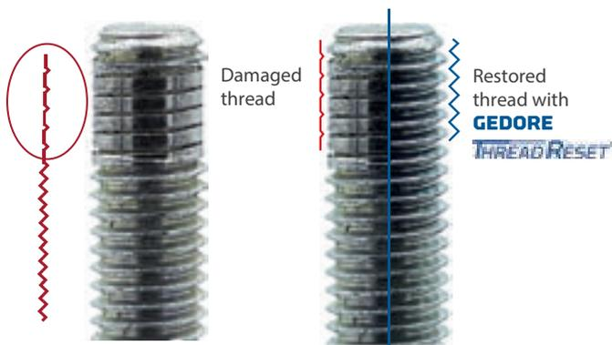
Image: Damaged thread in the upper area - functionality is no longer given
